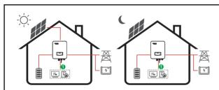
When the grid fails, the system will automatically switch to Back-Up mode. The back-up loads can be supplied by both PV and battery energy.
