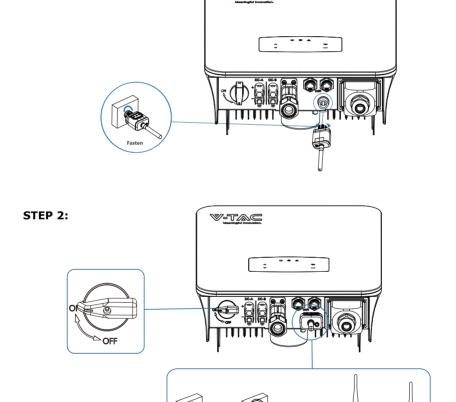
Turn on the DC switch and AC circuit breaker, and wait until the LED indicator on the monitoring module flashes, indicating that the monitoring module is successfully connected.
